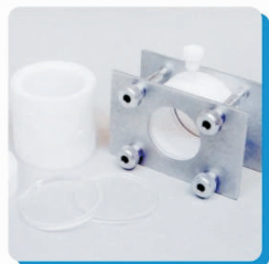
Demountable liquid cell, 10,20,40 mm optical path. Windows KBr, \text{CaF}_2 40 mm dia. Other window material may be ordered. Frame size 50x75 mm.
