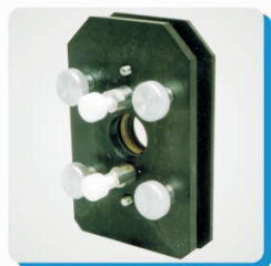
Demountable liquid cell, spacer set 0.1 to 1 mm (option 0.006 to 0.05 mm). Windows KBr, \text{CaF}_2 . Other window material may be ordered. Frame size 50x75 mm.
