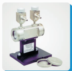
Gas cell, 100 mm optical path. Vacuum valves. Windows KBr, \text{CaF}_2 40 mm dia. Other window material may be ordered. Materials used: anodized glass, aluminium alloy, nickel plating, stainless steel.
