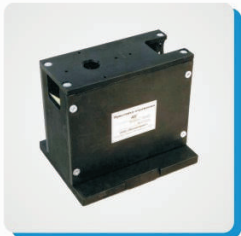
Specular reflectance accessory, 45° angle of incidence.
